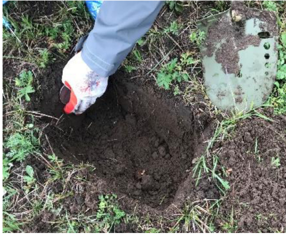
Fig. 4. Soil sample collection with a ring cutter.
