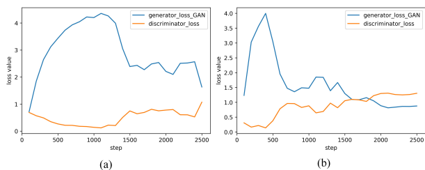
Fig. 5. Curves of loss functions with 2500 iterations. (a) AG-GAAN. (b) Pix2pix.
